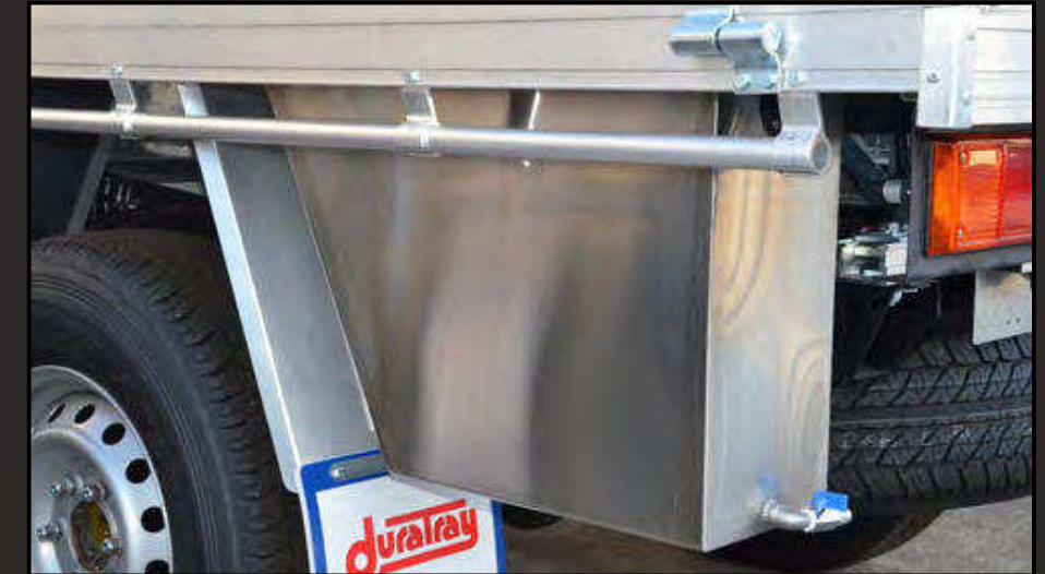
40L Stainless steel water tank
