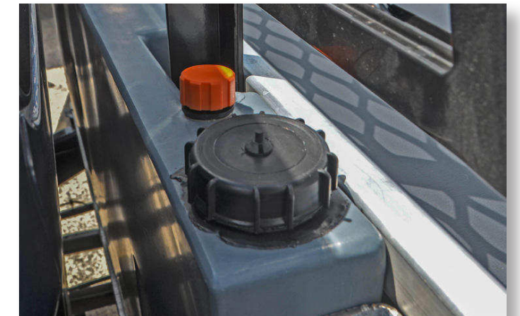
Tank fill point & breather
