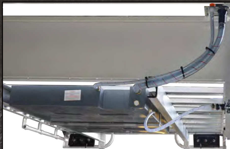
80L PVC slimline water tank mounts between tray and chassis
