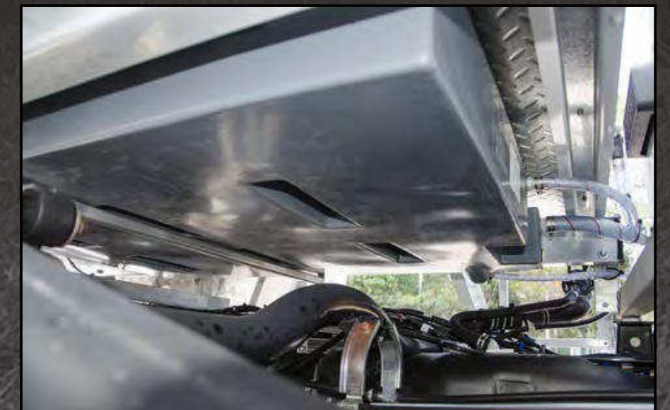
80L slimline tank size - 1080L x 830W x 115H
